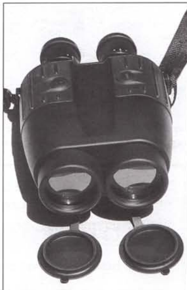
Above, author's new laser rangefinder — a Newcon Optik LRB 7x50. This rangefinder provided the author with accurate distance readings to over 1,000 yards.
